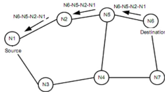
Fig 2: Route reply with route record with DSR
